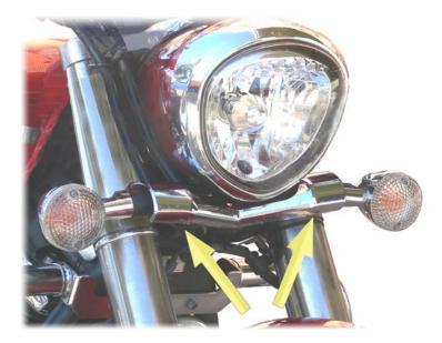
Once these screws have been removed, pull the trim towards the front to release it from its central elastic anchor.
